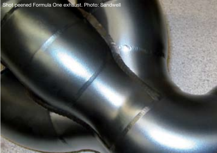
Shot peened Formula One exhaust. Photo: Sandwell
