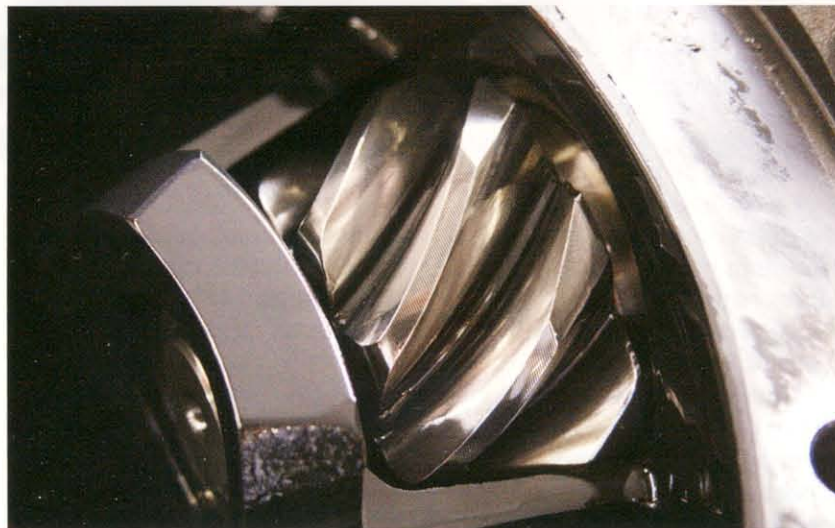
The pinion does not show any type of wear or heat discoloration. All the more impressive considering that the locker, ring, and pinion all have more than 5,000 laps on them.
