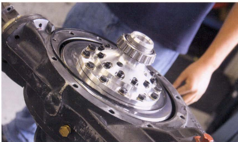
The RF85 metal treatment has been applied to this particular asphalt Late Model but it will also work on the spool-type or rearends that Dirt Late Models utilize.
