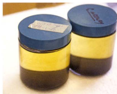
Tiger Rear Ends performed many tests on the oil to ensure the viscosity of the oil was not breaking down. This particular oil has more than 250 laps on it.
